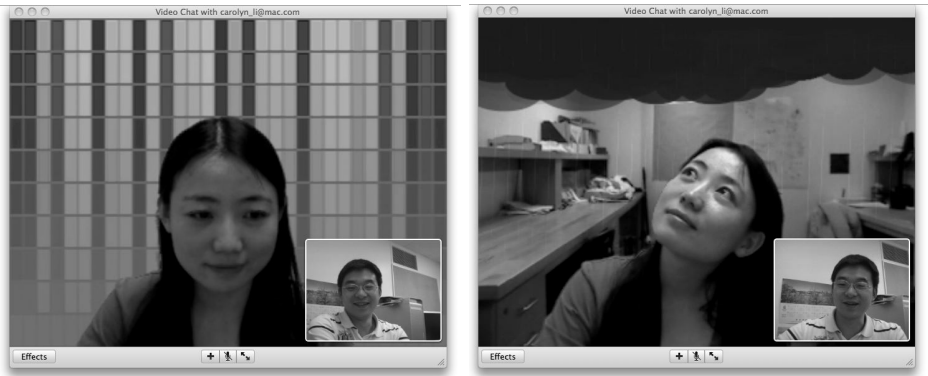
Fig. 7. Supraliminal backdrops. On the left, colored blocks. On the right, the users’s office superimposed with rain clouds. The animations are driven either by pseudo-random bits or ciphertext, estimable by the recipient.
